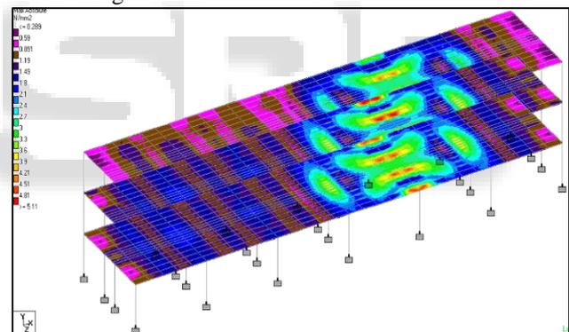
Fig. 7: Stress diagram of slab showing increase in stress (Red colour) at the location of floating column.
