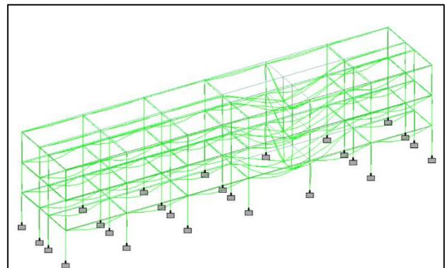
Fig. 5: Deflection Diagram of whole framed structure.
