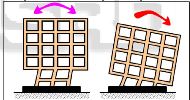
Fig. 1: Tilt of building due to floating column.
