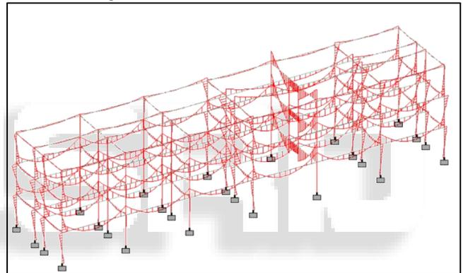
Fig. 4: Bending Moment Diagram in the frame where floating column is different.
