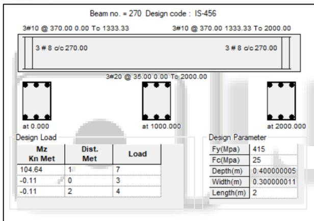
Fig 6: Reinforcement detailing of the beam below floating column.
