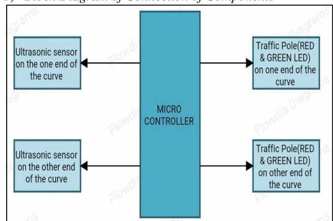
Ultrasonic sensor has four pins. They are +5V, VCC, GND, Trig pin and Echo pin. Here the Trigger pin is the Output pin and the Echo pin is the Input pin. Ultrasonic sensor send the signal in the form of pulse from the trigger pin. When the signal hits the object it will reflected back and received by echo pin. Microcontroller UNO processes this data and operates the LED which is connected to the output pin of the Microcontroller Arduino UNO.
