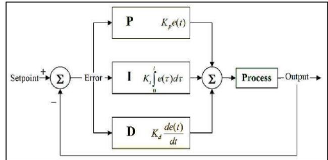
The proportional value determines the reaction to the current error, the integral value determines the reaction based on the sum of recent error, and derivative value determines the reaction based on the rate at which the error has been changing. The weighted sum of these three actions is used to adjust the process via a control element such as the position of a control valve or the power supply of heating element. Thus, a PID controller has the general form:
