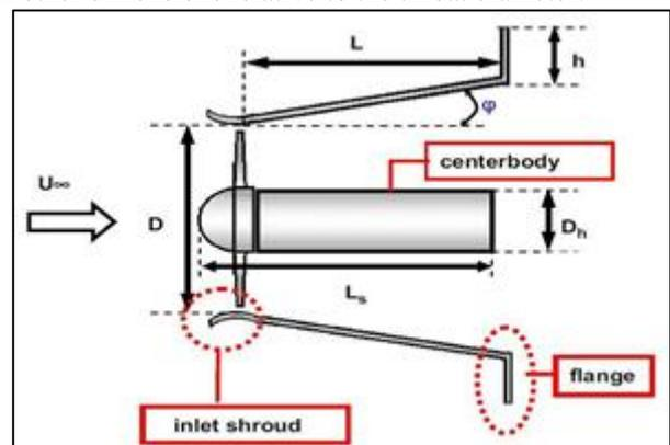
Fig. 5: Diagram of shroud with Dimension  $D=0.65$  m
