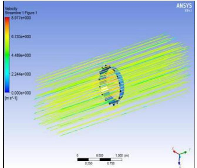
Fig. 29: Velocity contour of bumped diffuser without brim
