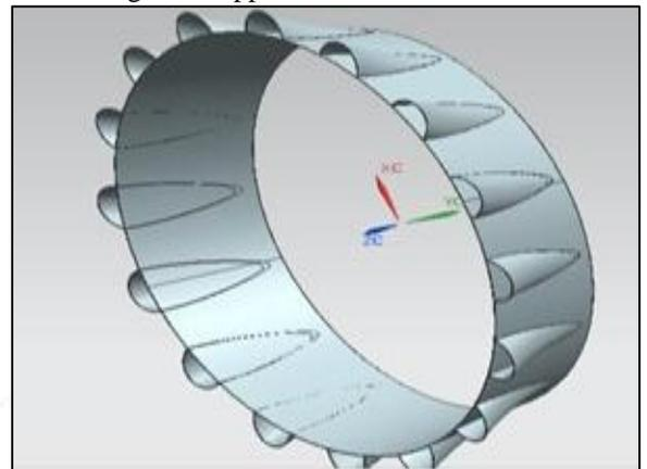
Fig. 11: Bumped diffuser without brim
