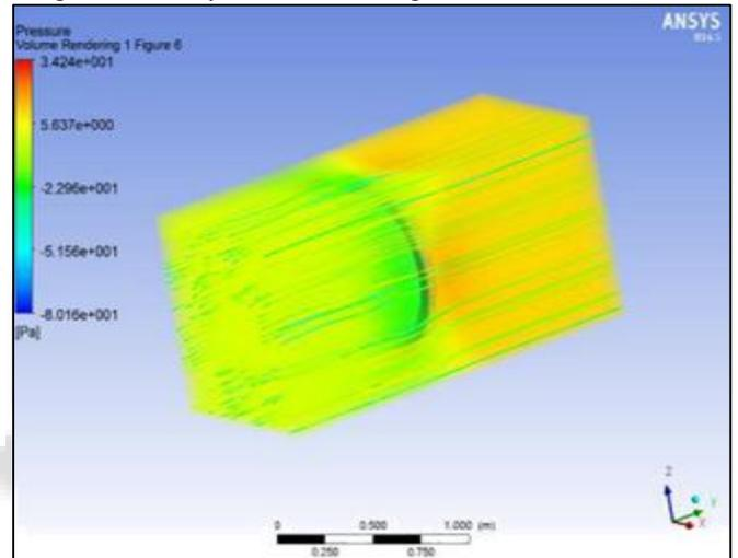
Fig.18: pressure contour of straight diffuser with brim
