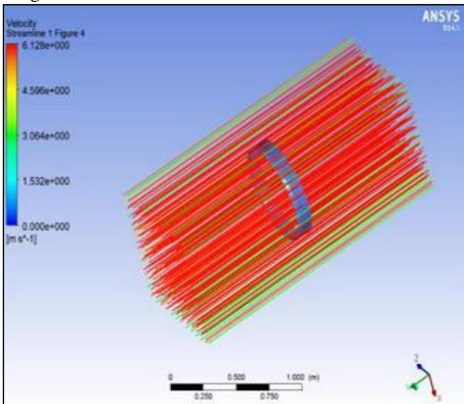
Fig. 21: Velocity contour of curved diffuser without brim
