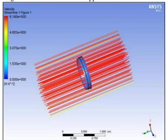
Fig. 25: Velocity contour of Stepped diffuser without brim
