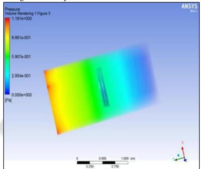
Fig. 24: Pressure contour of Stepped diffuser without brim
