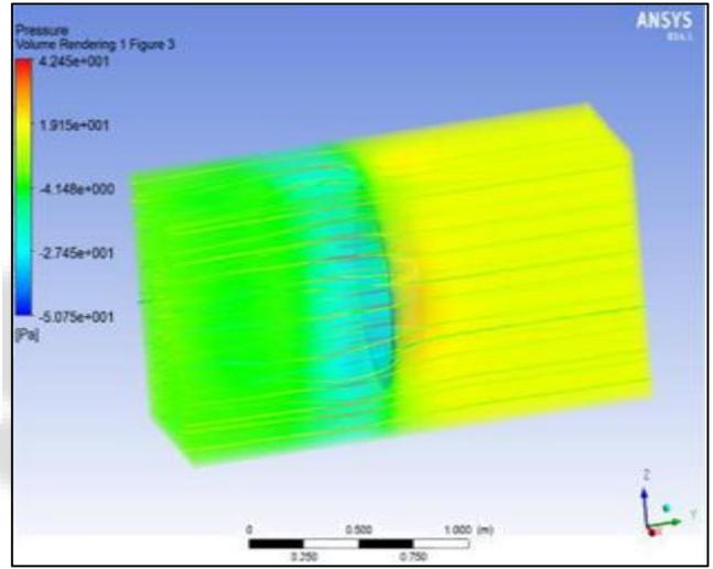
Fig. 30: Pressure contour of bumped diffuser with brim
