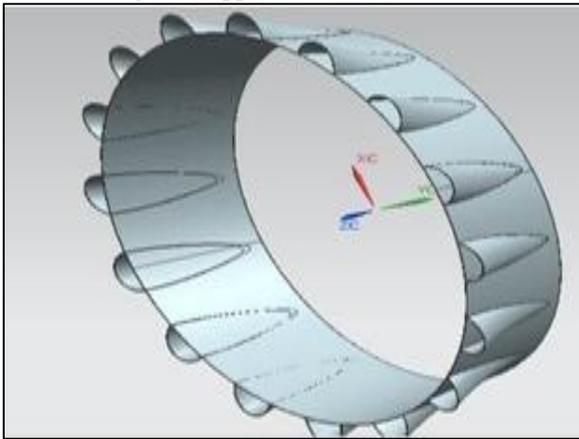
Fig.15: Bumped diffuser with brim
