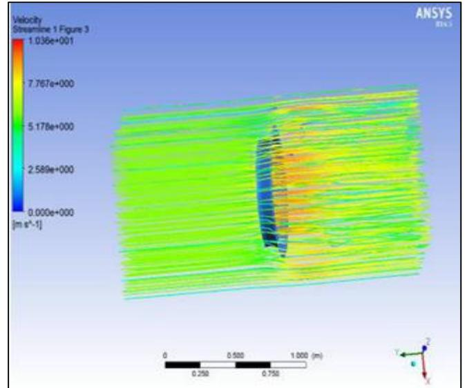
Fig. 23: Velocity contour of curved diffuser with brim
