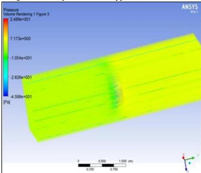
Fig. 28: Pressure contour of bumped diffuser without brim
