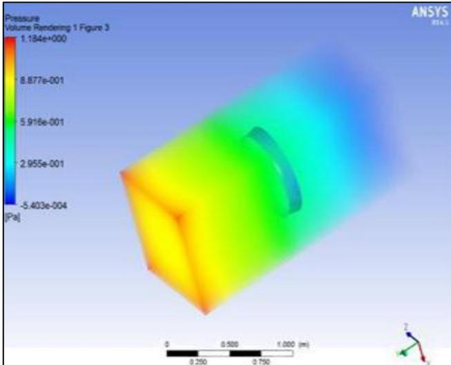
Fig. 20: Pressure contour of curved diffuser without brim
