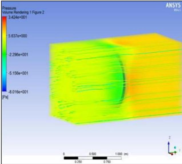
Fig. 26: Pressure contour of Stepped diffuser with brim
