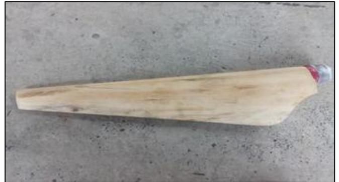
Fig. 3: NACA 63(2)215 Airfoil blade
