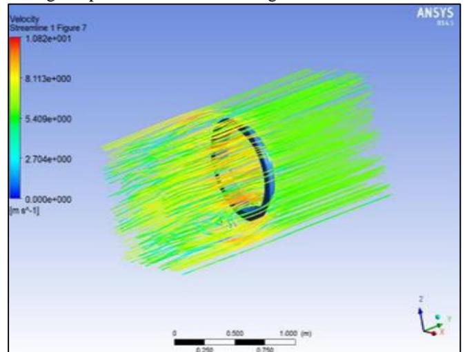
Fig.19: Velocity contour of straight diffuser with brim
