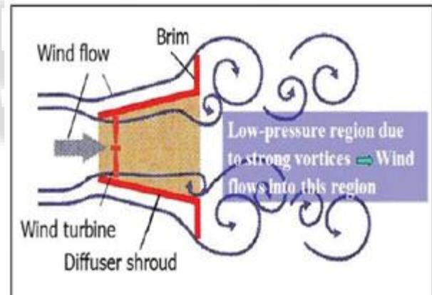
Fig. 1: Principle of increase in the mass flow rate of the air
