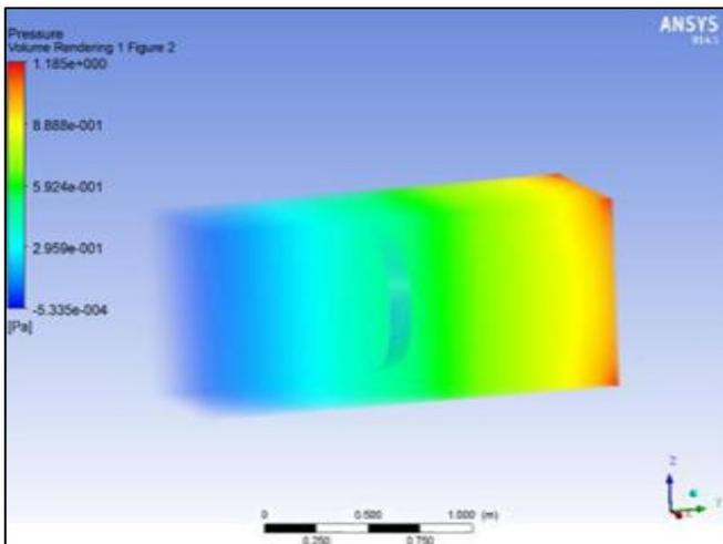
Fig. 16: pressure contour of straight diffuser without brim
