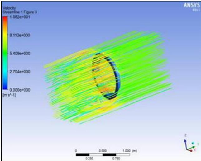
Fig. 27: Velocity contour of Stepped diffuser with brim
