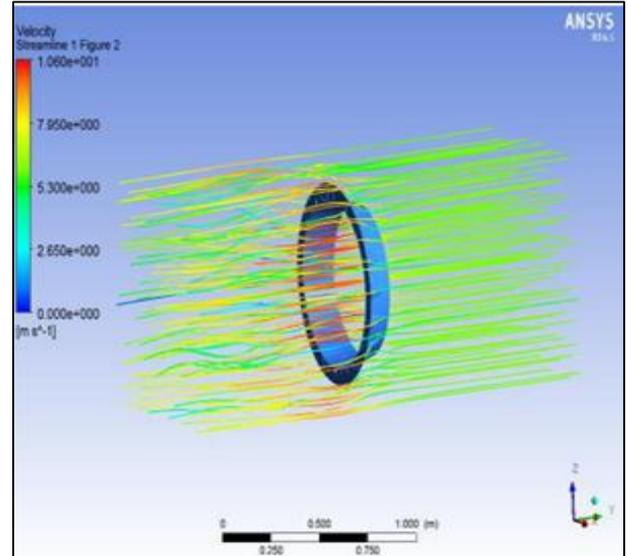
Fig. 31: Velocity contour of bumped diffuser with brim
