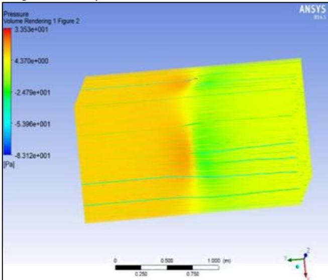
Fig. 22: Pressure contour of curved diffuser with brim
