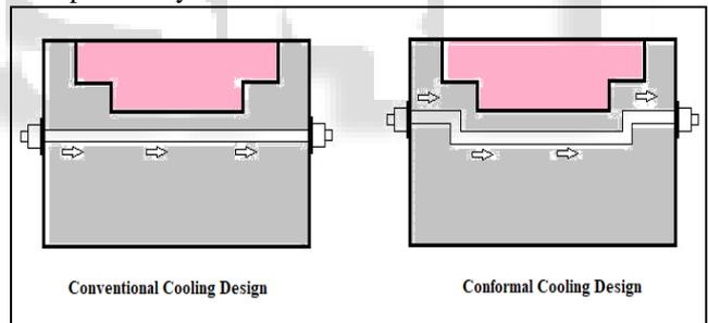
Fig. 3: Conventional and Conformal Cooling Channels
