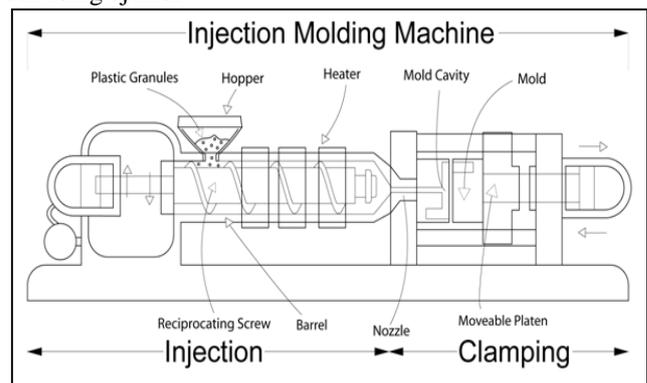
Fig. 1: Injection Moulding Process
