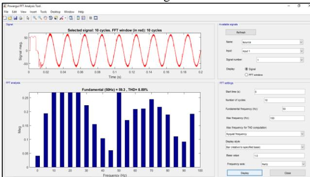
Fig. 4.4: Fast Fourier Transform and Total Harmonic Distortion of the input signal
