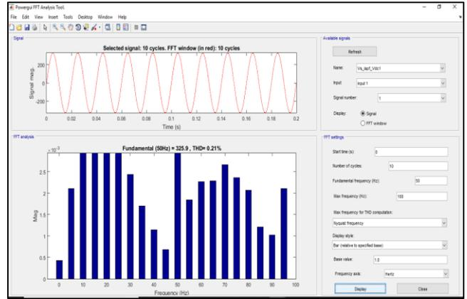
Fig. 4.5: Fast Fourier Transform and Total Harmonic Distortion of the APF output signal
