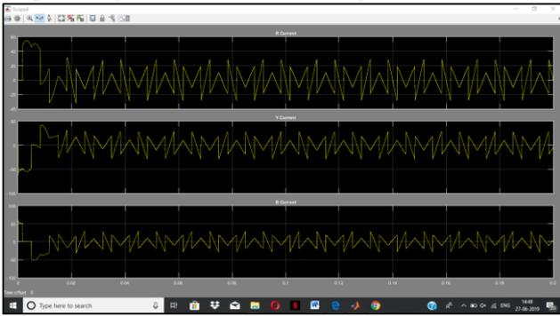
Fig. 4.1: Compensating current for RYB phase
