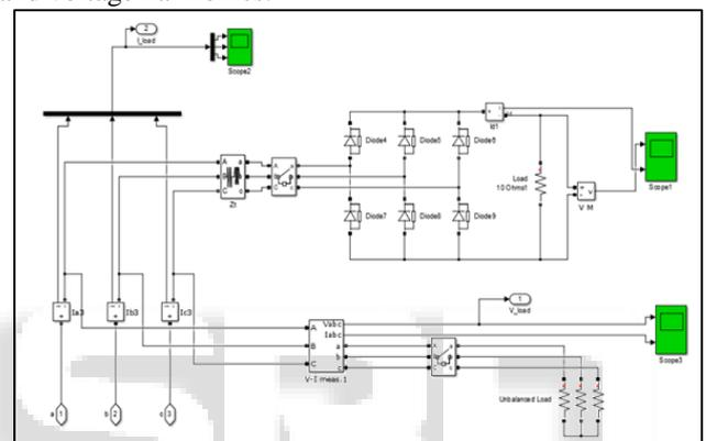
Fig. 3.4: Non-linear load model
