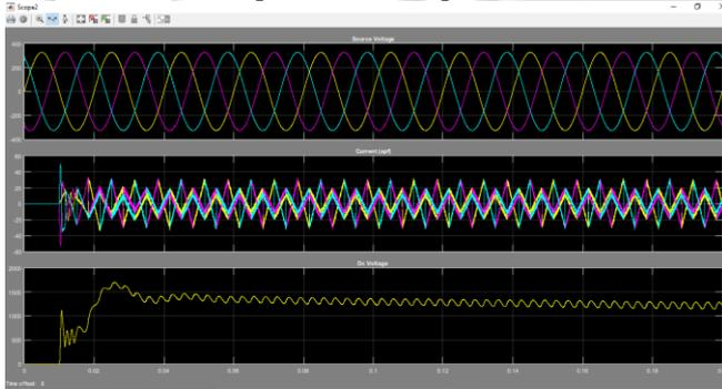
Fig. 4.3: Source voltage, APF system Current output, DC voltage
