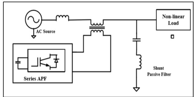
Fig. 3.3: Series APF with Shunt Connected Passive Filter
