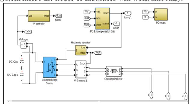
Fig. 3.5: Shunt active filter model
