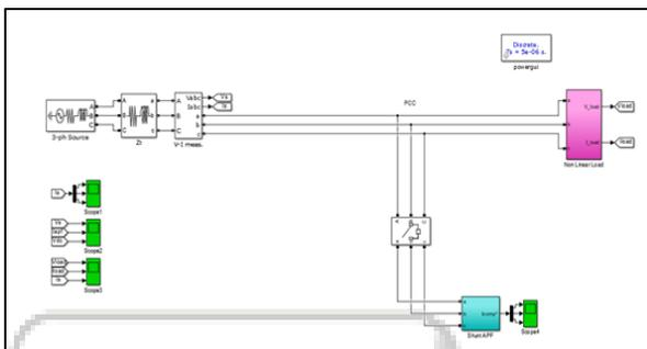
Fig. 3.1: Simulink model of shunt active power filter
