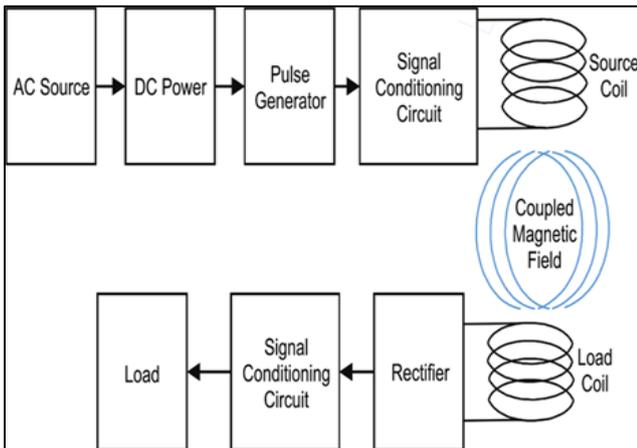
Fig. 6: Block Diagram of WPT Circuitry
