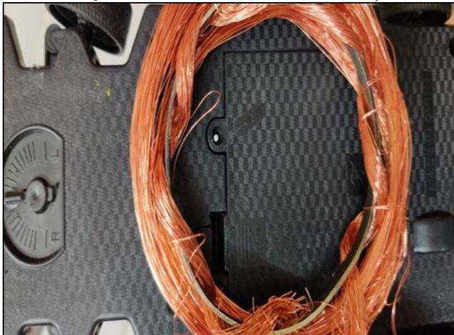
Fig. 7: receiving coil attached to bottom end of model
