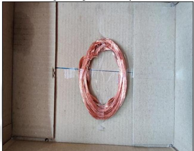
Fig. 9: secondary coil places under Cardboard box representing underground
