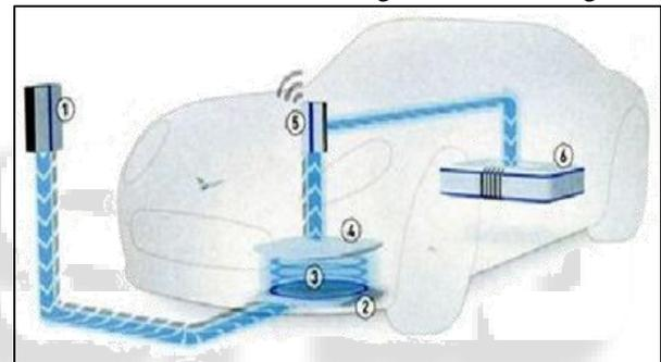
Fig. 1 A basic Wireless Charging Unit for a Car.
