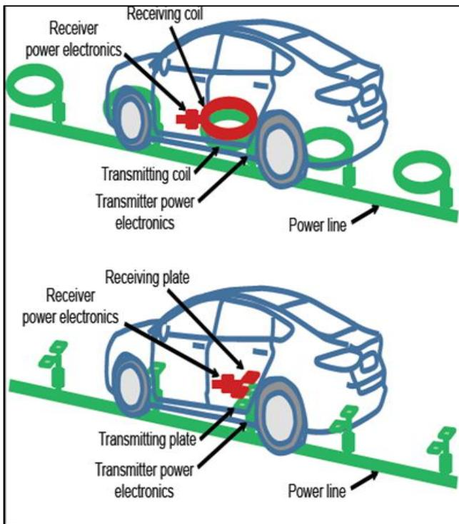
Fig. 2: Underground Wireless Charging Unit for a EV Car using coils & Fig. 3 Underground Wireless Charging Unit for a EV Car using Transmission plates.
