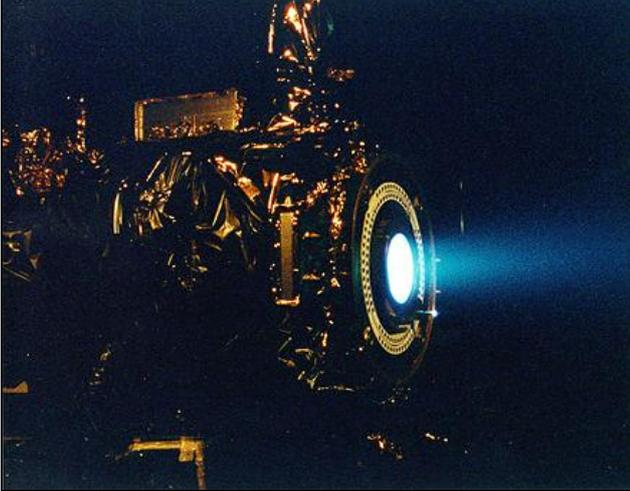
This is the actual image of the test firing of the ion thrusters for the Deep Space spacecraft at the Jet propulsion Laboratory (NASA)
