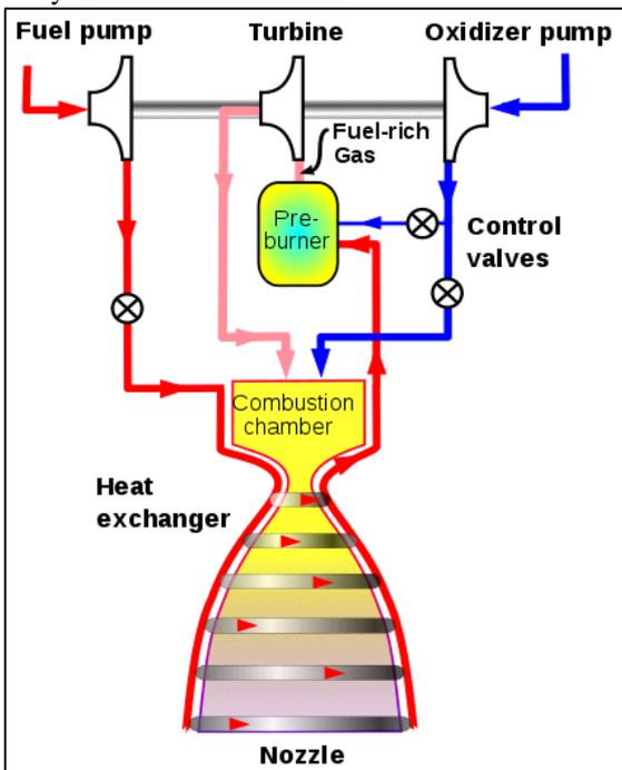
Fig. 3: Staged combustion
