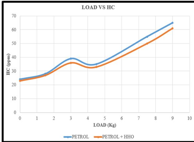
Fig. 6: Load vs HC Emission
