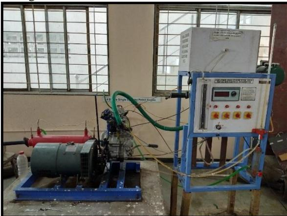
Fig. 2: Four stroke petrol engine test rig
