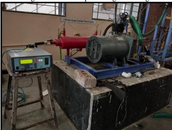
Fig. 3: Test rig with Petrol analyzer
