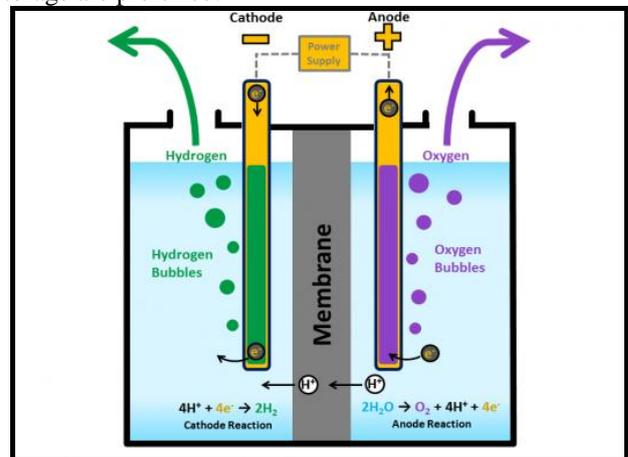
Fig. 1: Electrolysis of Water
