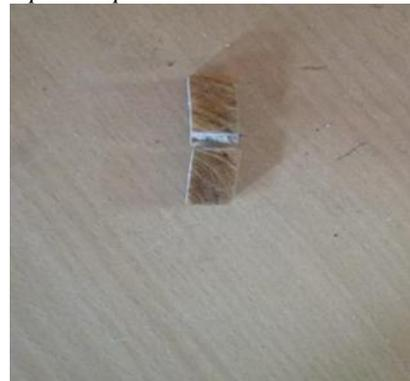
Fig. 6.35: Jute fiber Charpy test specimen
