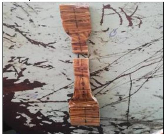
Fig. 6.1: Jute Tensile Specimen (After test)
