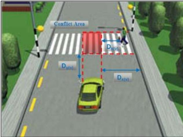
Fig. 1: Showing Position of Vehicle and Pedestrian with respect to Conflict Zone
