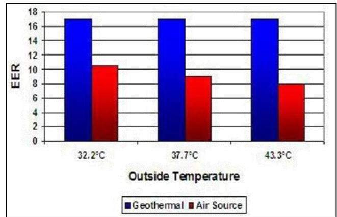
Fig. 6.1: Comparison Geothermal vs. Air Source Cooling.
