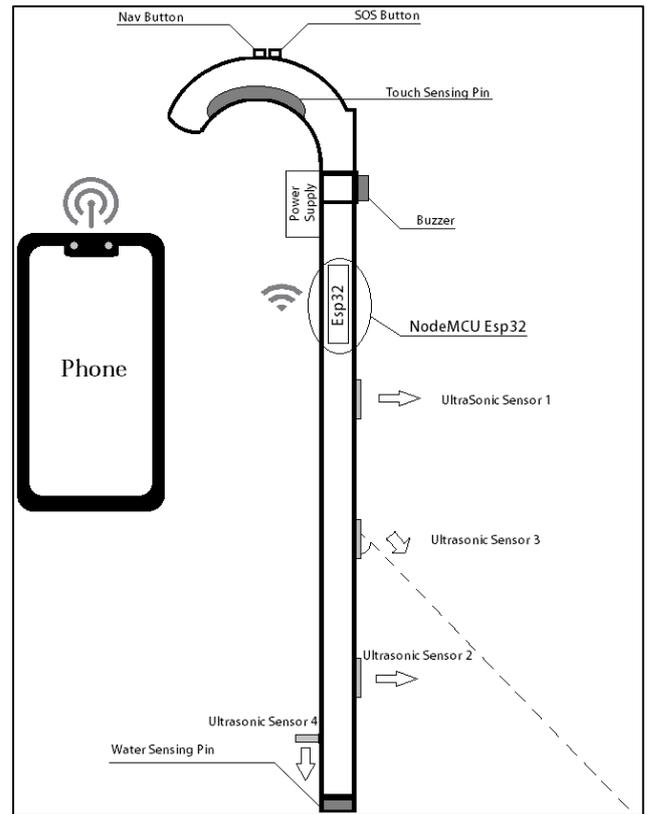
Fig. 2: Schematic Diagram of Smart Walking Stick
