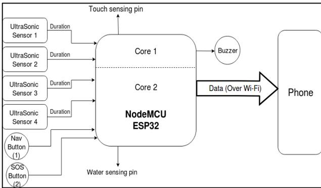
Fig. 1: Block Diagram of Smart Walking Stick
