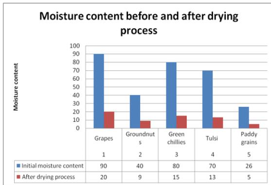
Fig. 12: Moisture content before and after drying process of crop dryer unit
