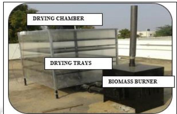
Fig. 6: Hardware model of drying chamber with biomass burner
