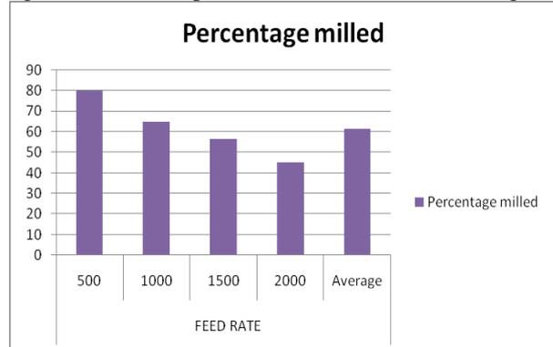
Fig. 11: Percentage of Milled paddy crop drains Vs feedrate in dehussing unit
