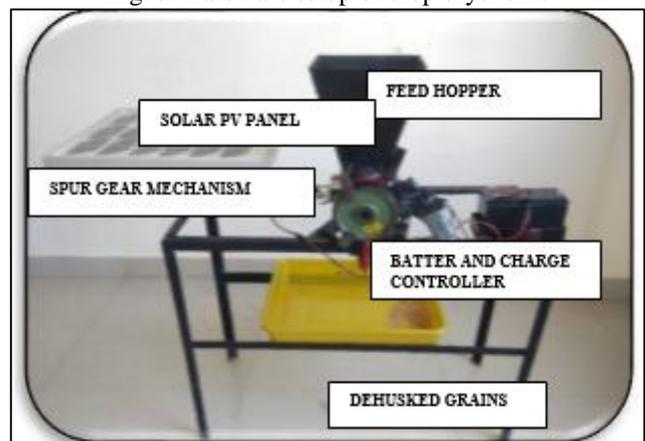
Fig. 8: Hardware setup of solar dehusking unit
