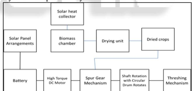
Fig. 1: Basic block diagram of solar crop dryer with Dehusking unit
