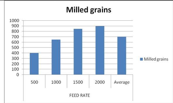
Fig. 8: Milled paddy crop drains Vs feedrate in dehussing unit
