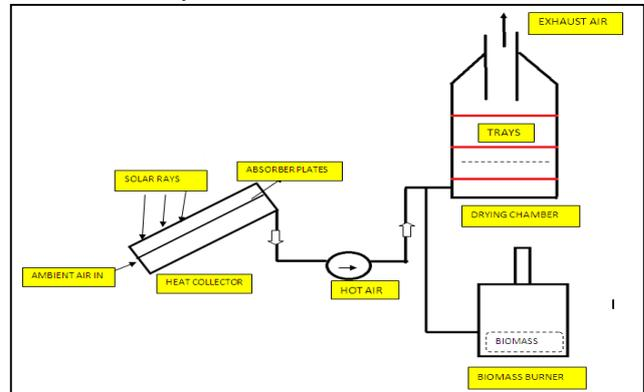
Fig. 2: Working of Solar & biomass integrated crop dryer
