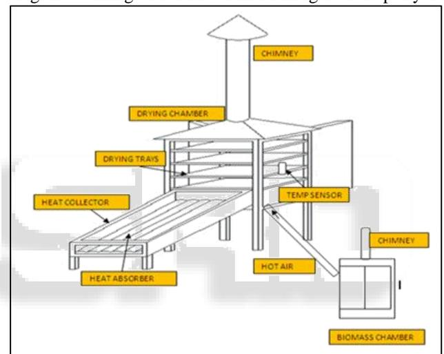
Fig. 3: Solar & biomass integrated crop dryer layout
