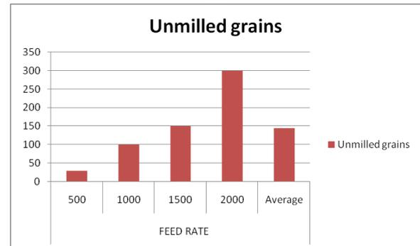
Fig. 9: Unmilled paddy crop drains Vs feedrate in dehussing unit
