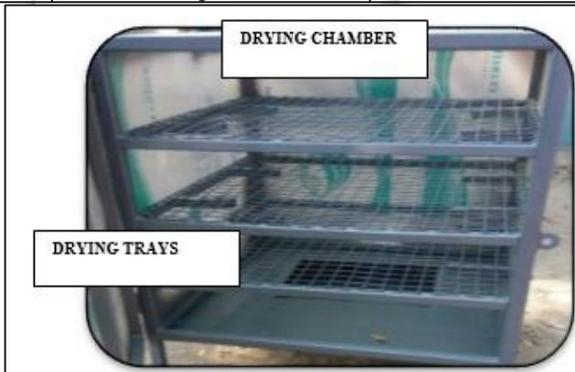
Fig. 4: Hardware model of drying chamber
