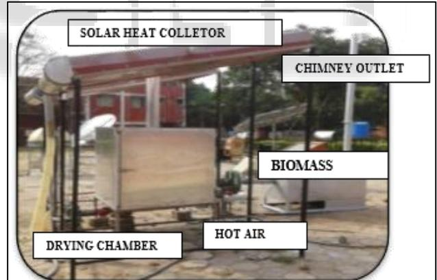
Fig. 7: Hardware setup of crop dryer unit
