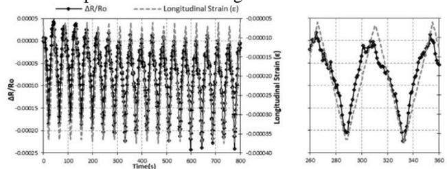
Graph. 4.2 Strain sensing for Load 625.500kN
