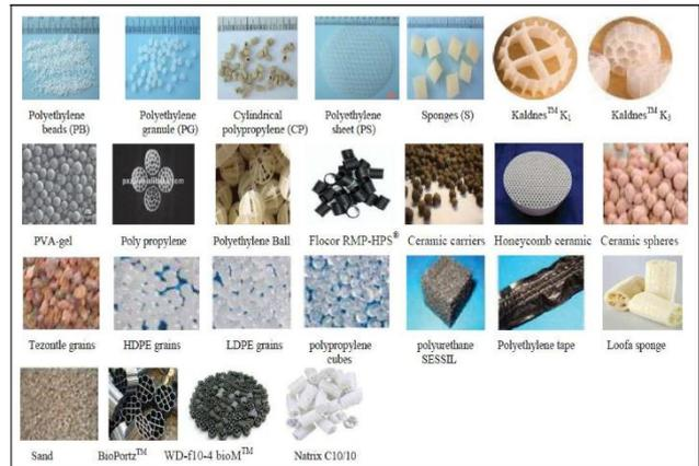
The physical appearance of the media used in attached growth processes
