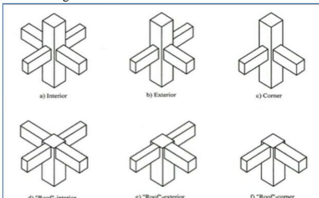
Fig. 2: Types of joints
