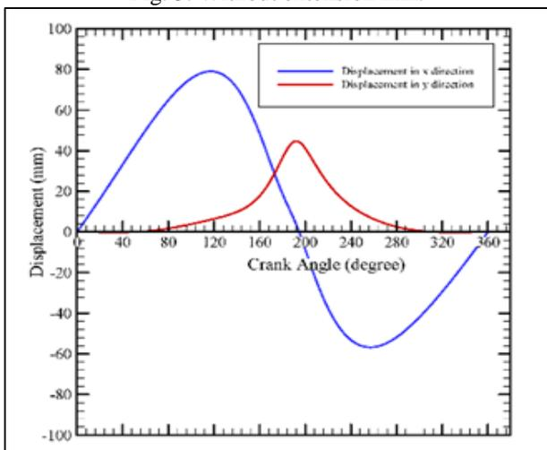
Fig. 4: x and y displacement with respect to crank angle
