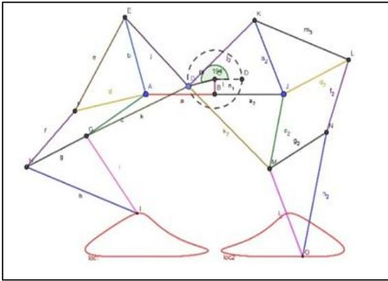
Fig. 2: Path traced by front and back leg
