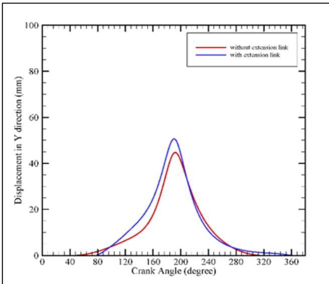
Fig. 8: Comparison of y displacement without and with extension link
