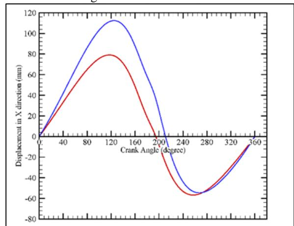
Fig. 7: Comparison of x displacement without and with extension link
