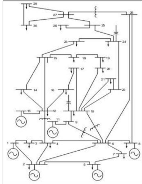
Fig. 4: Single line diagram for IEEE 30 bus system
