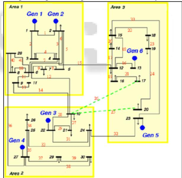
Fig. 5: IEEE 30 bus system Configuration.
