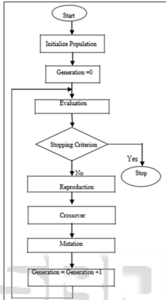
Fig. 3: Genetic Algorithm Flowchart.
