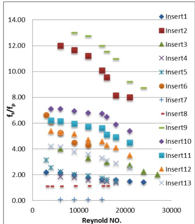
Fig. 4: Variation of Friction factor enhancement Ratio ( $f_i/f_p$ ) Ratio Vs Reynold Number for different types of inserts
