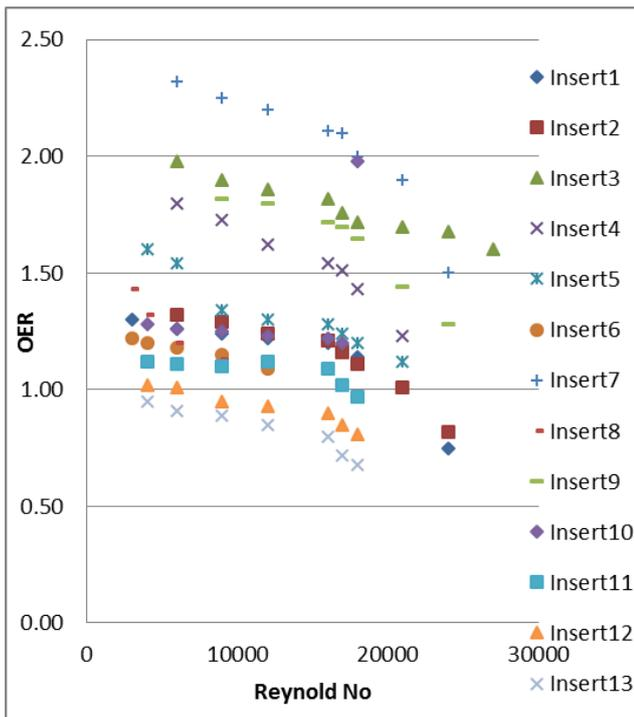
Fig. 5: Variation of Overall enhancement Ratio (OER) Vs Reynold number for different types of inserts.
