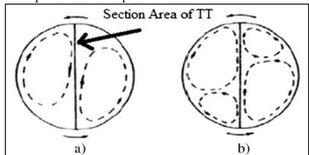
Fig. 1: Secondary induced flow pattern by TT [4]
