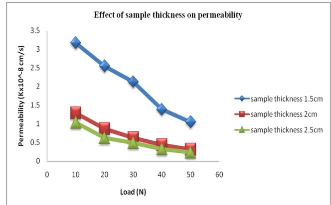
Graph 2: Permeability – Sample thickness curve
