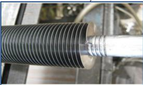
Fig. 5: Knurled finned tube (Aluminium)
