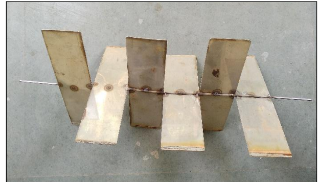
Fig. 2.1: Flow Divider without dimpled type baffles
