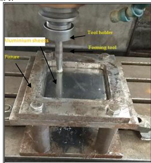
Fig. 1: Shows SPIF process experimental setup and
