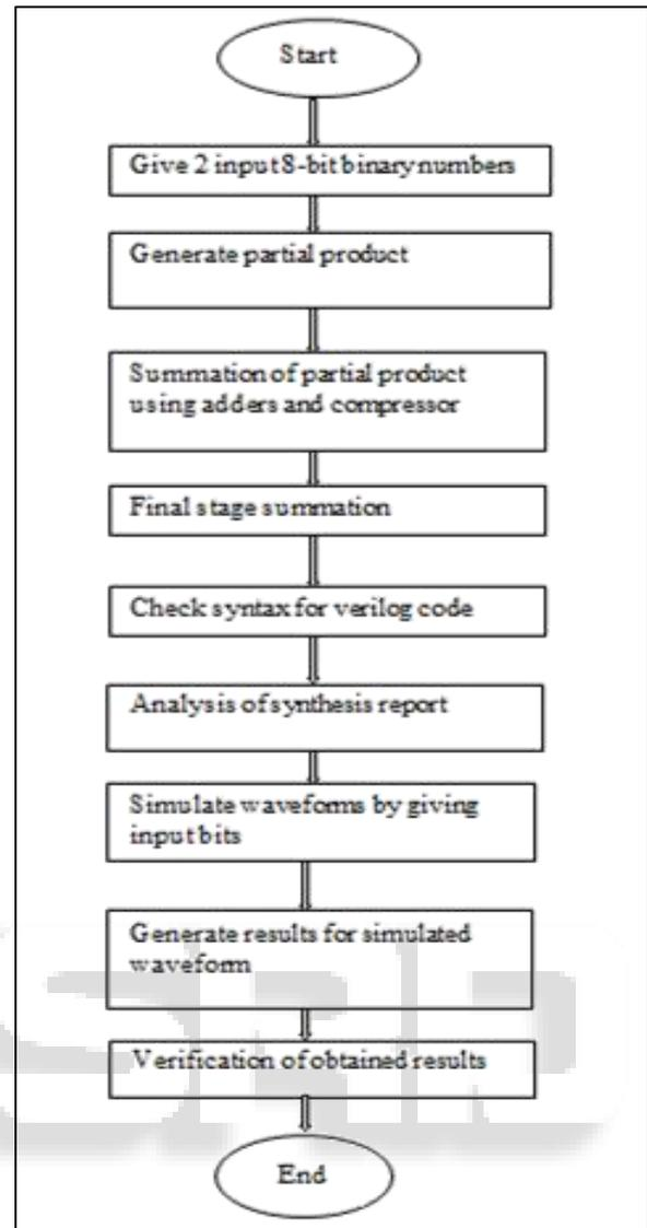
Fig. 5: Proposed algorithm of Wallace tree using compressor technique
