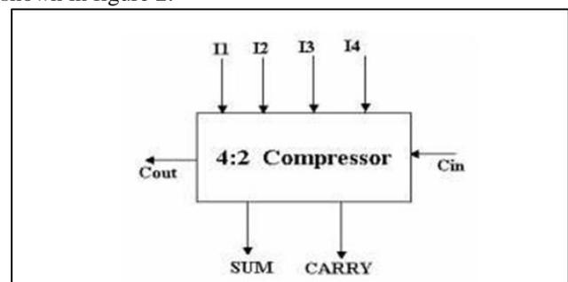
Fig. 1: Block diagram of 4:2 compressor
