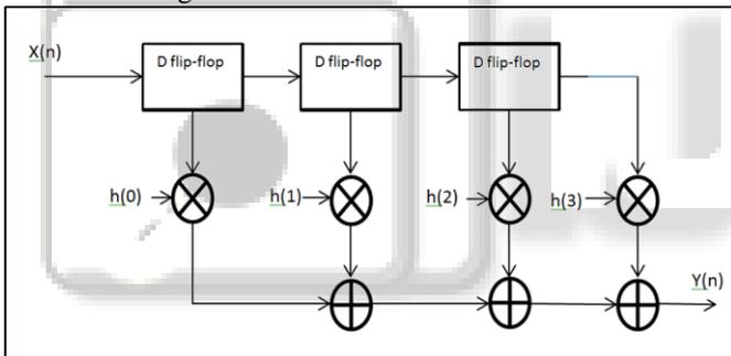
Fig. 3: Block diagram of FIR filter
