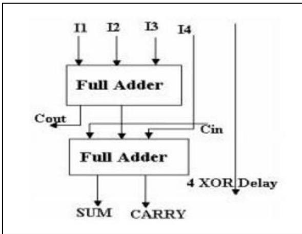
Fig. 2: Compressor design using Full adders
