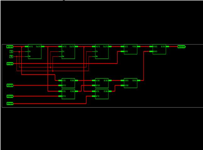
Fig. 7: FIR filter based on wallace tree
