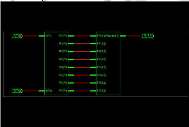
Fig. 8: Wallace tree multiplier based on compressor
