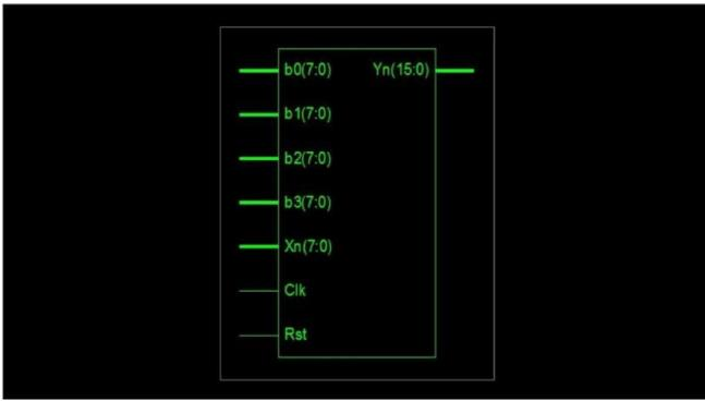
Fig. 6: Main RTL schematic
