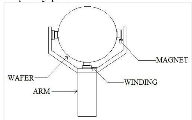
Fig. 1: Schematic diagram of wafer gripping mechanism.
