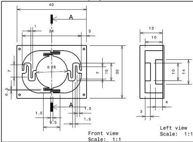
Fig. 6: 2D drawing of gripper module showing front and left side views. All dimensions are in mm.
