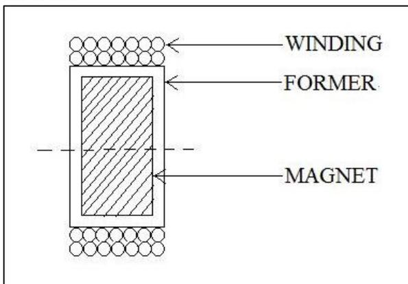
Fig. 3: Schematic diagram of the solenoid
