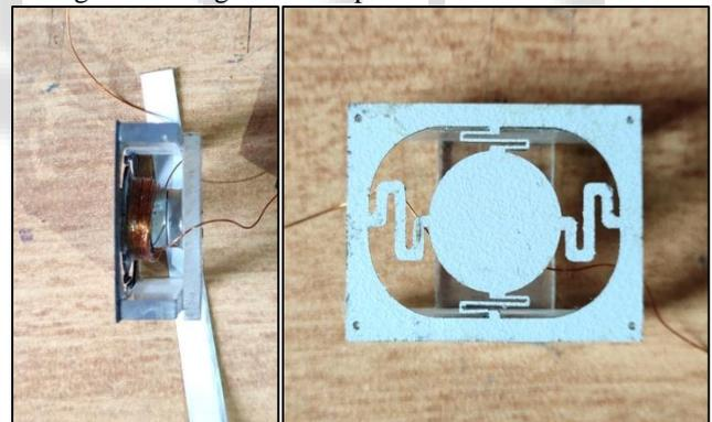
Fig. 8: (left to right) Fig 8: (a) Right side view of the fabricated gripper module.
