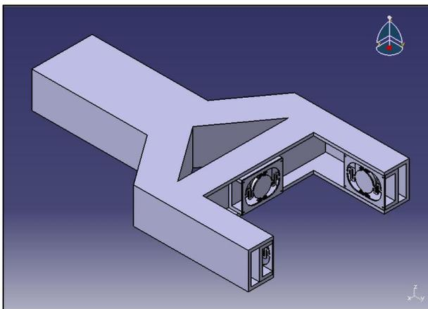
Fig. 7: 3D model of the wafer gripping mechanism
