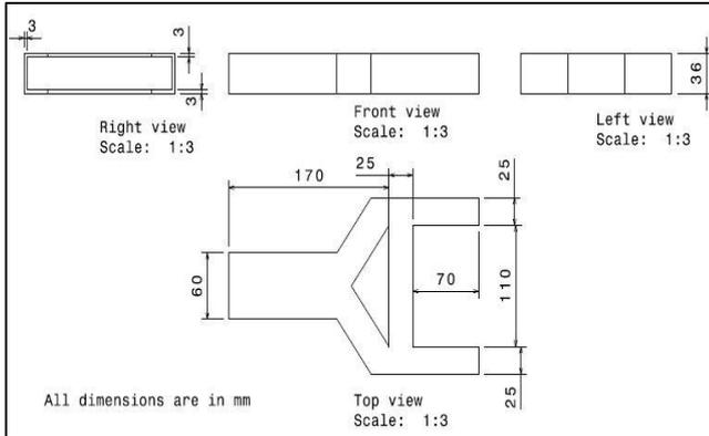
Fig. 2: 2D drawing of the arm showing all views
