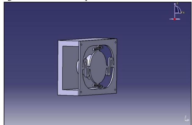
Fig. 5: 3D model of the gripper module
