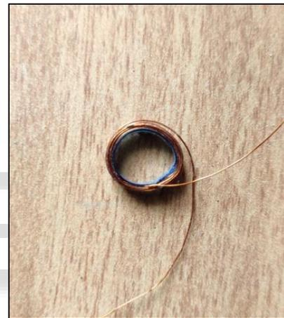
Fig. 4: Image of the fabricated solenoid coil
