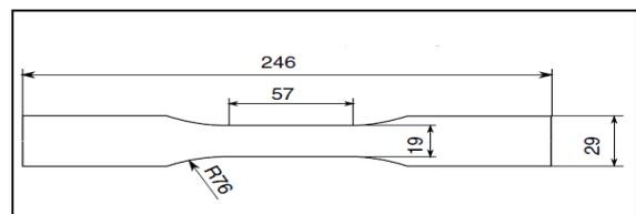
Fig. 5: Tensile test specimen as per ASTM D638
