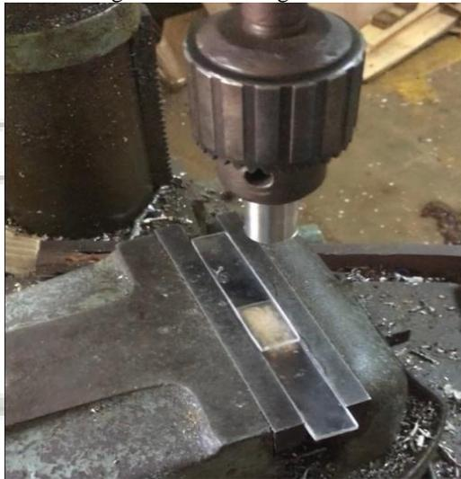
Fig. 2: FSSW setup on pillar drilling machine
