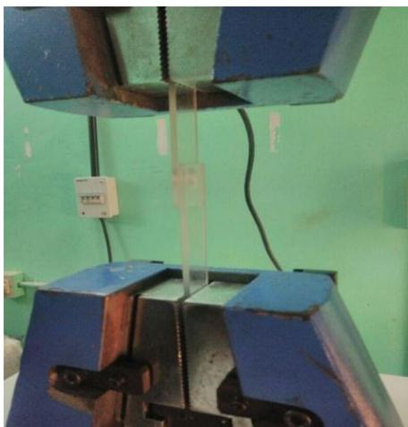
Fig. 7: Close-up view of specimen in UTM
