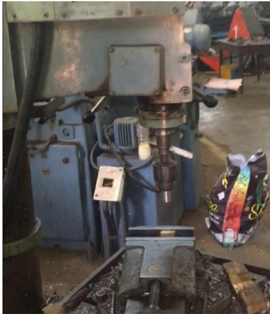
Fig. 1: Pillar drilling machine
