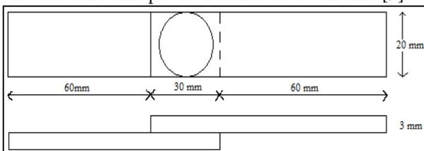
Fig. 3: Dimensions of the workpiece for FSSW
