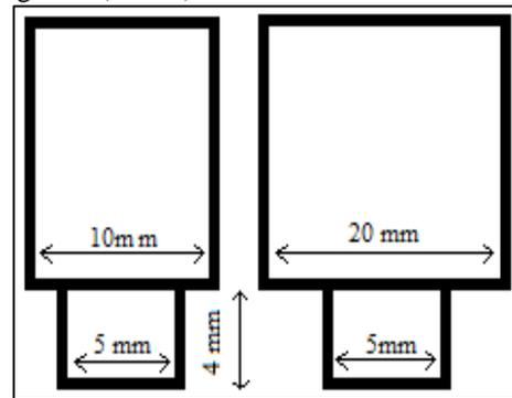
Fig. 4: Schematic of tools (T2 and T1 respectively)
