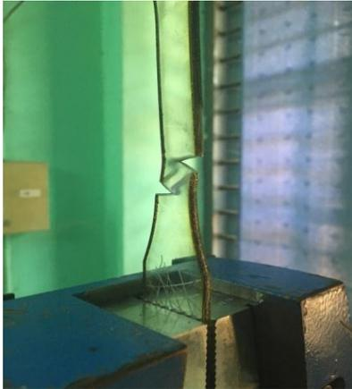
Fig. 6: Tensile specimen after tensile test
