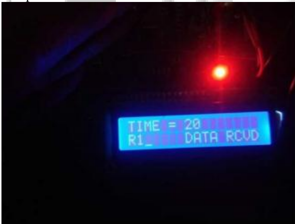
Fig. 4: Update the Time when Emergency Vehicles Detected with Road Number
