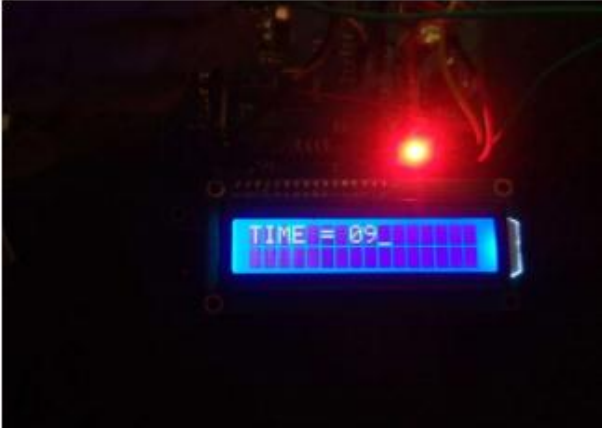
Fig. 3: Passing time for Vehicles in normal mode Synchronization of initial time for signal junction when there is no emergency vehicle in any of the roads. This time is constant for every road until any emergency vehicles get detected by the camera.
