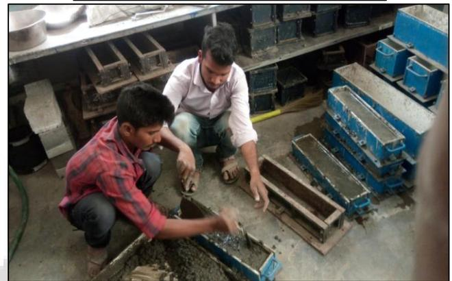
Fig. 2: Casting Cube and Beam
