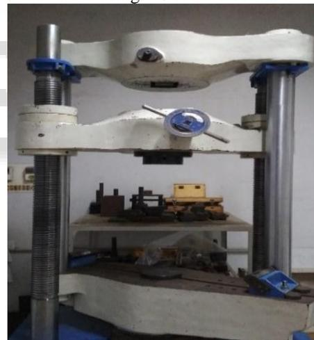
Fig 6: Universal Testing Machine
