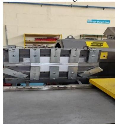
Fig 1: Friction stir welding machine
