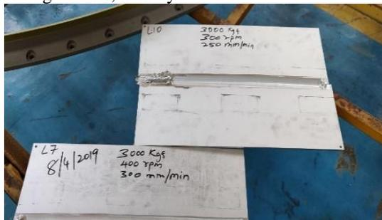
Fig 5: Welded specimen
