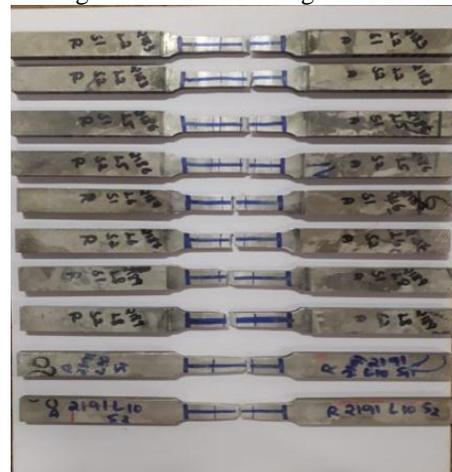
Fig 7: Specimens after tensile test
