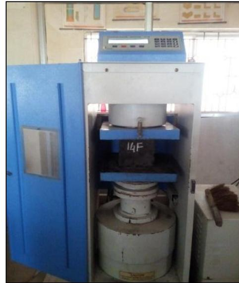
Fig. 3: compressive strength Test
