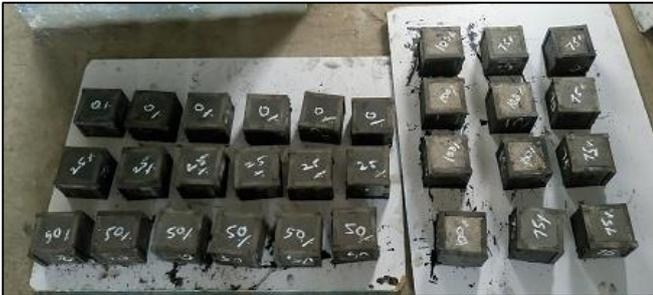
Fig. 1: Casted Mortar Cube Specimens
