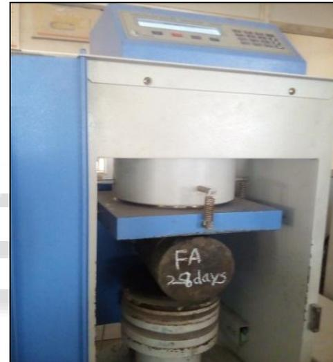
Fig. 4: split tensile strength Test
