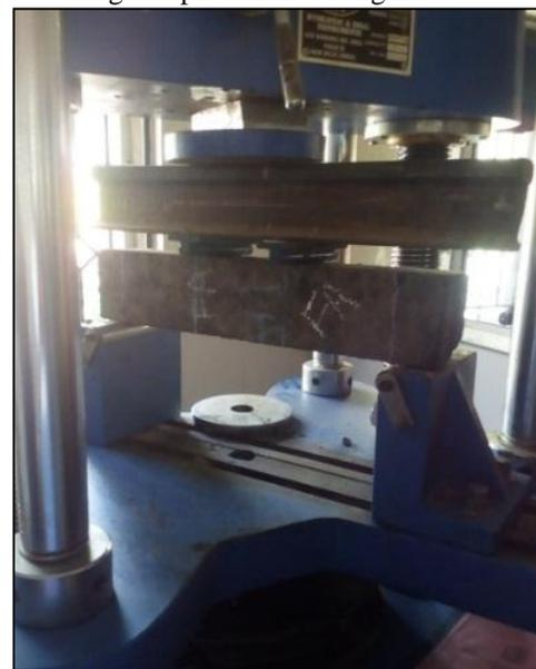
Fig. 5: Flexural Strength Test
