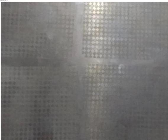
Fig. 4: Circular grid is made on the lower side of titanium grade 2 sheet.
