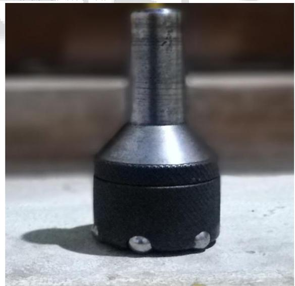
Fig. 2: Multi point incremental forming tool (patent protected)
