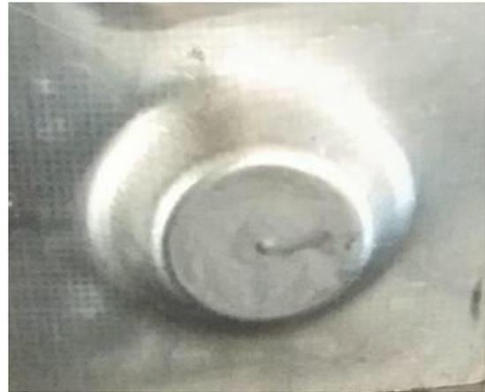
Fig. 5: Conical frustum shape is formed on the sheet.
