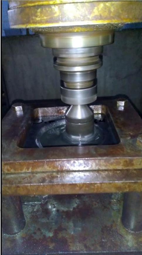
Fig. 3: Multi point incremental forming process.
