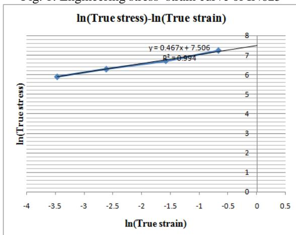
Fig. 2: ln (true stress) versus ln (true strain) graph
