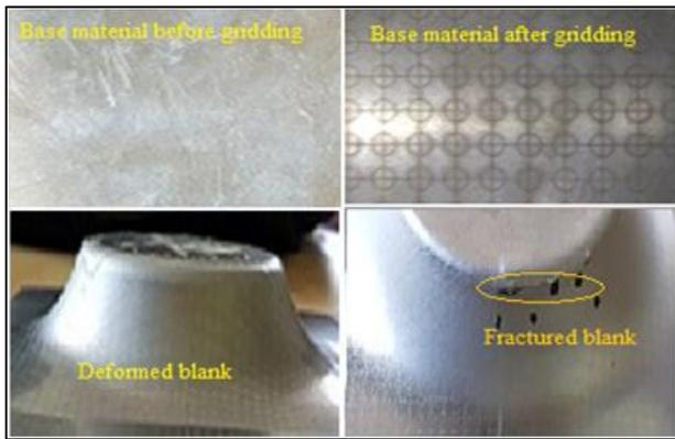
Fig. 3: Shows (a) SPIF process experimental setup and (b) SPIF process operations of Inconel 625 sheets blanks.
