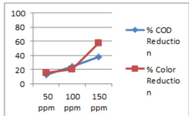
Fig. 4: Removal of COD and Color and dose indicates of Hydrogen Peroxide
