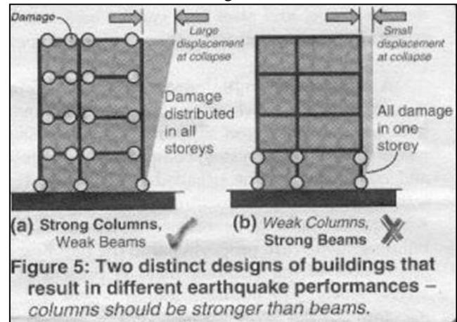
Figure 5: Two distinct designs of buildings that result in different earthquake performances – columns should be stronger than beams.
