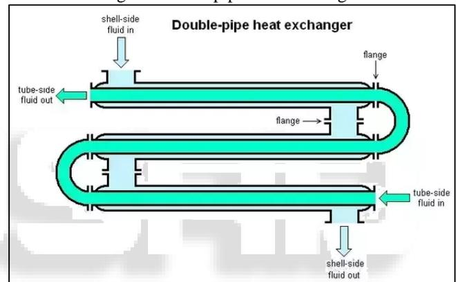
Fig. 4: U-type double pipe heat exchanger
