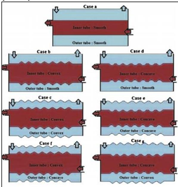
Fig. 1: Different corrugated tubes in a DPHE
