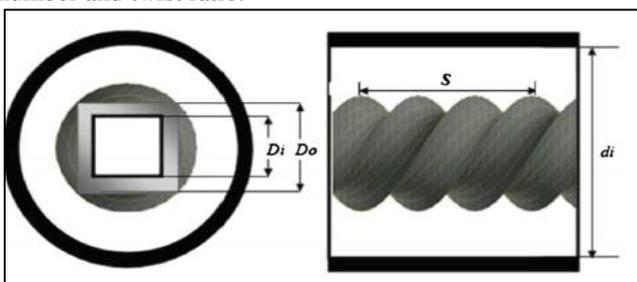
Fig. 2: Twisted inner tube of the DPHE
