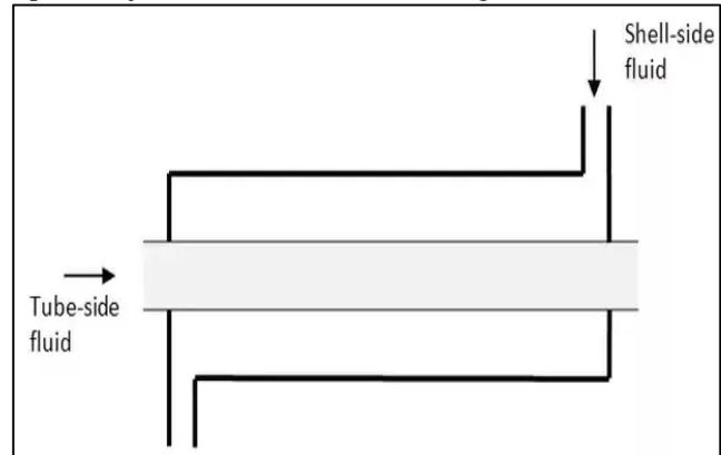
Fig. 3: Double pipe heat exchanger
