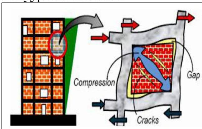
Fig. 1: Behavior of the infill wall as a strut member
