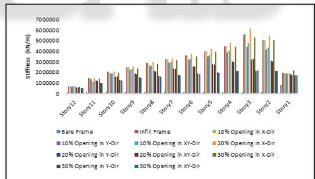
Fig. 3.2: Storey Stiffness in Y direction (kN/m)
