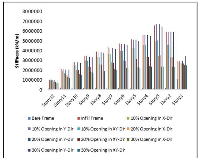
Fig. 3.1: Storey Stiffness in X direction (kN/m)
