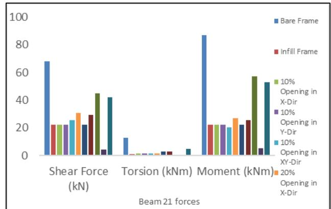
Fig. 5: Shear Force, torsion, moments in B21
