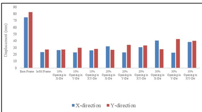
Fig. 3: Maximum Lateral Displacement (mm)
