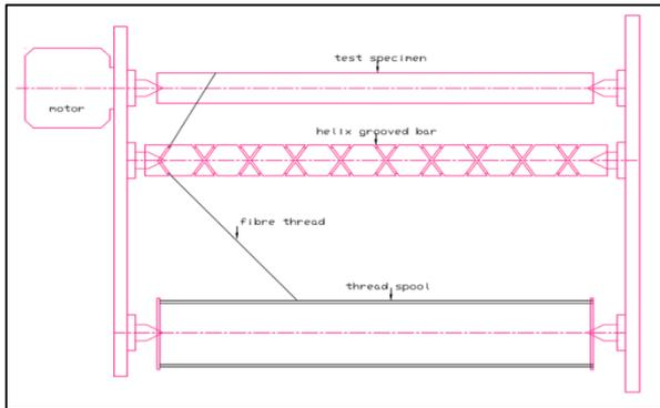
Fig. 2: Proposed design of filament winding machine.
