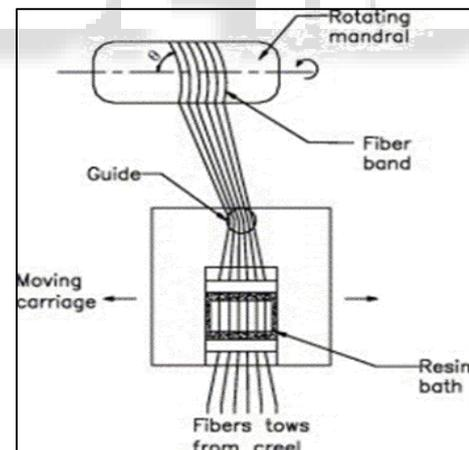
Fig. 1: Schematic of Filament winding[7]
