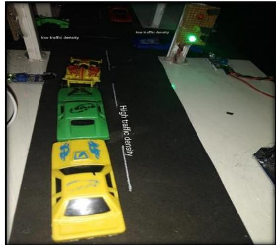
Fig. 4.3: Green signal provided to road 4 for more time due to high traffic
