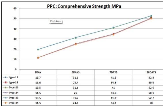
Fig. 2: Sample compared with PPC grade
