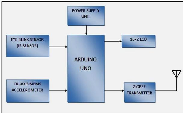
Fig. 1: Transmitter end of the system
