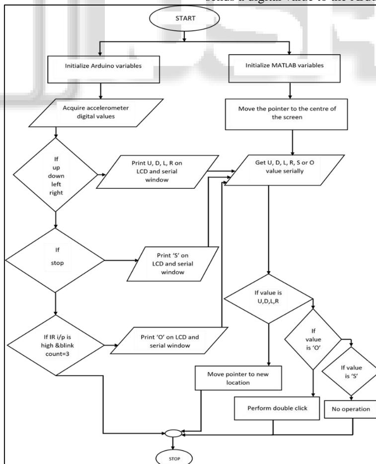
Fig. 3: Flowchart indicating the system working
