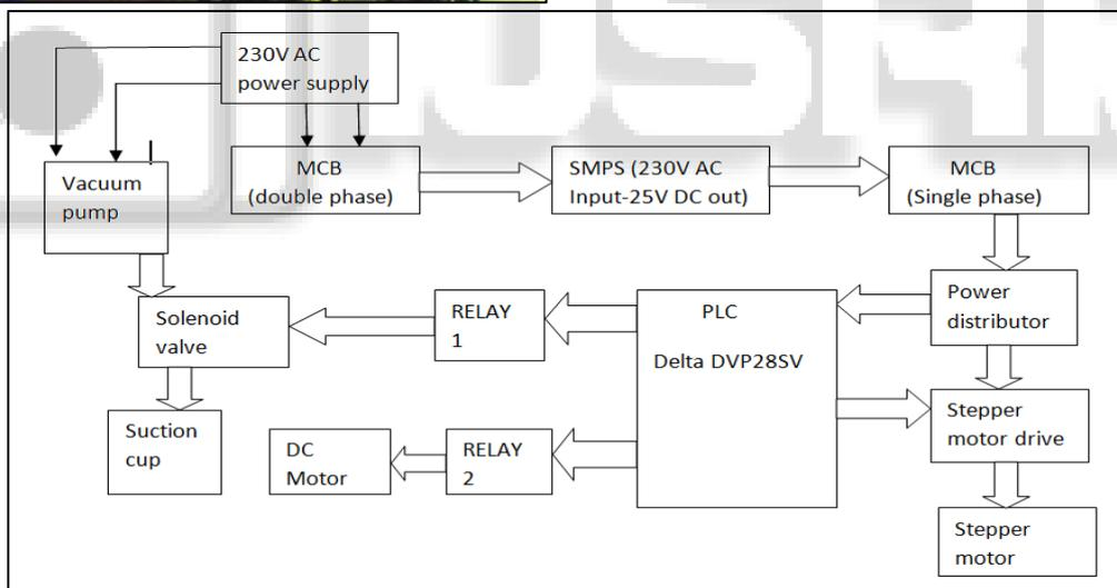
Fig. 10: Block diagram of control panel.
