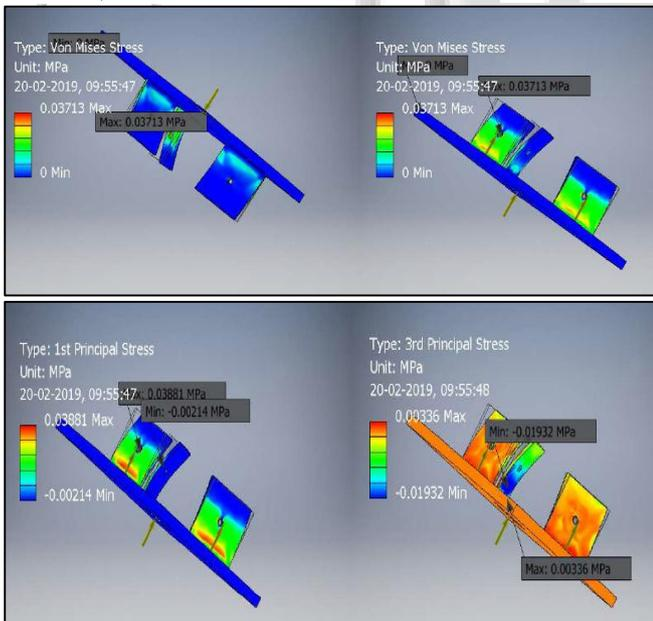
Fig. 3: 3D model of base plate with Von mises stress analysis
