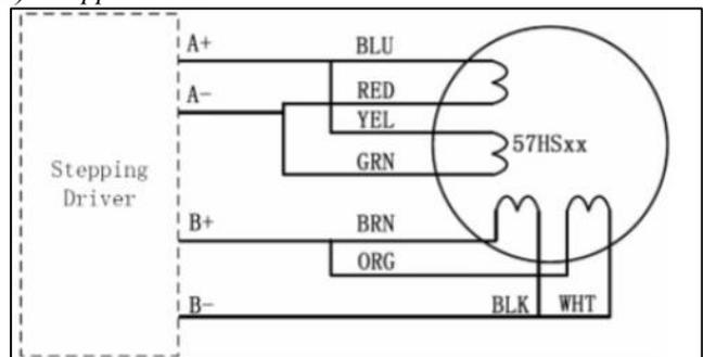
Fig. 11: Stepper motor to stepper drive parallel connection
