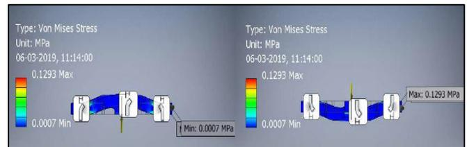
Fig 5: von mises stress analysis of end effector
