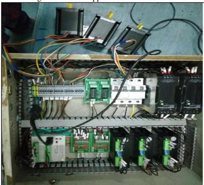
Fig. 13: Actual Interfacing of control panel with stepper motor
