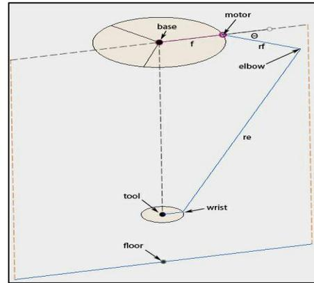
Fig. 14: Robot mechanism dimensions
