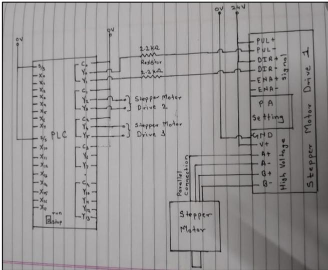
Fig. 12: PLC to stepper motor connections
