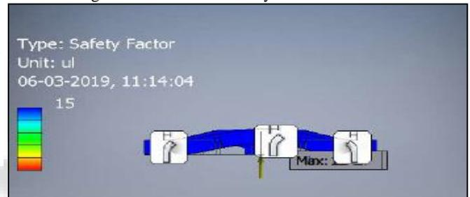
Fig. 6: Safety factor analysis of End effector.
