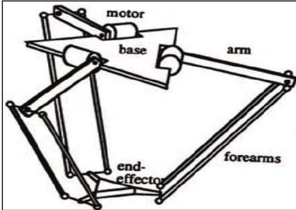
Fig. 2: Structure of delta robot
