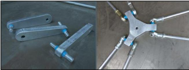
Fig. 8: Fabricated parts using plasma cutting machine
