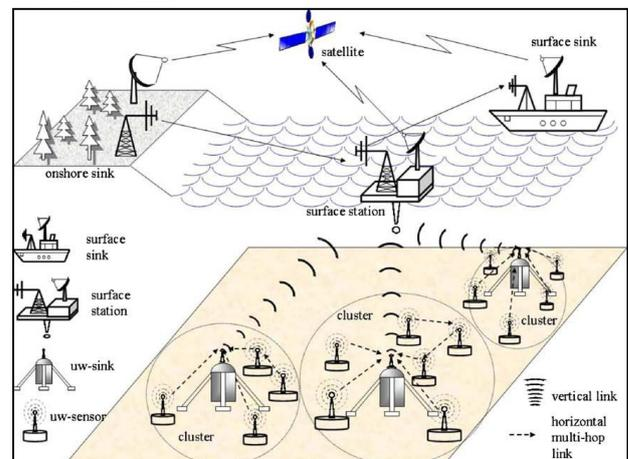
Fig. 1: Architecture of 2D UWSNs
