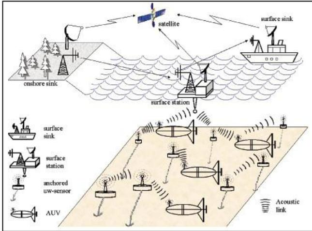
Fig. 2: Architecture of 3D UWSNs
