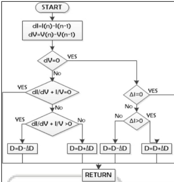
Fig. 3: Incremental Conductance flowchart
