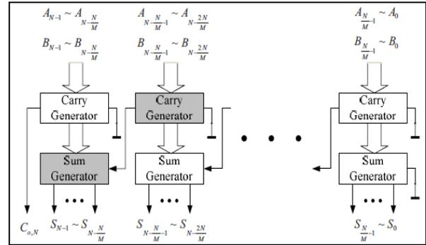
Fig. 3.6: Circuit diagram of the ETA-II adder.
