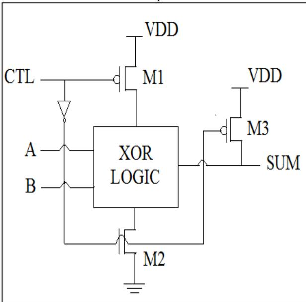
Fig. 4: Schematic diagram of modified XOR gate [11]
