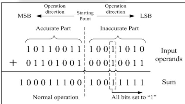
Fig. 1: Error Tolerant Adder [11]
