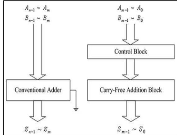
Fig. 2: Architecture diagram of ETA [11]
