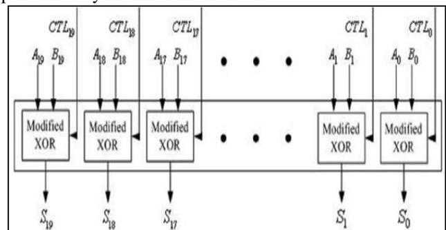
Fig. 3: Architecture diagram of carry free addition block [11]
