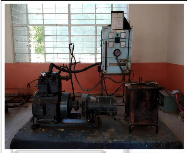
The objective of this paper is to reduce the waste heat from engine, to implement eco-friendly power generation method for domestic and commercial use and to improve the overall efficiency of the engine. This can be done by connecting thermoelectric generator at the exhaust of the twin cylinder engine. The efficiency of the twin cylinder engine is approximately 45% and this can be increased by connecting TEG at the exhaust of twin cylinder engine.
