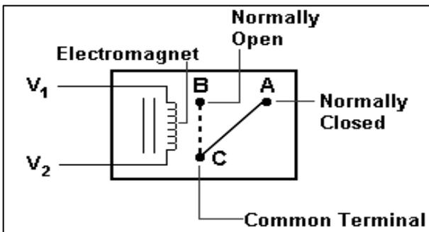
A relay acts as electrically operated switch. Current flows through the coil of the relay creates a magnetic field which attracts a lever and changes the switch contacts. The coil current can be on or off ,so relay has two switch positions and they are double throw (changeover) switches.
