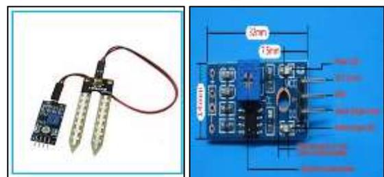
FC-28 soil moisture sensor is a simple breakout for measuring the moisture in a soil and similar materials. The soil moisture sensor is user friendly. The two large exposed pads function as probes for the sensor, which acts as a variable resistor.
