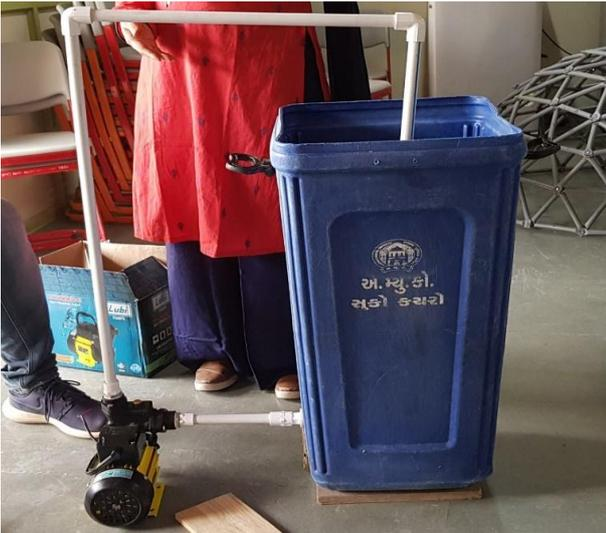
The model consist of a 0.5 HP pump attached to the a drum of 50 litres capacity through Pipes.
