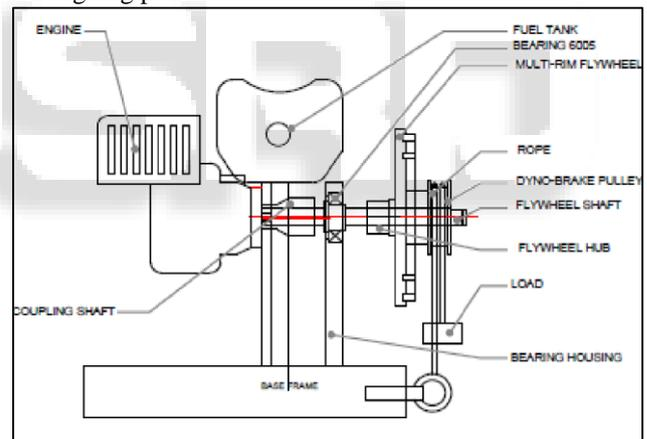
Fig. 3: Schematic of conventional flywheel test rig
