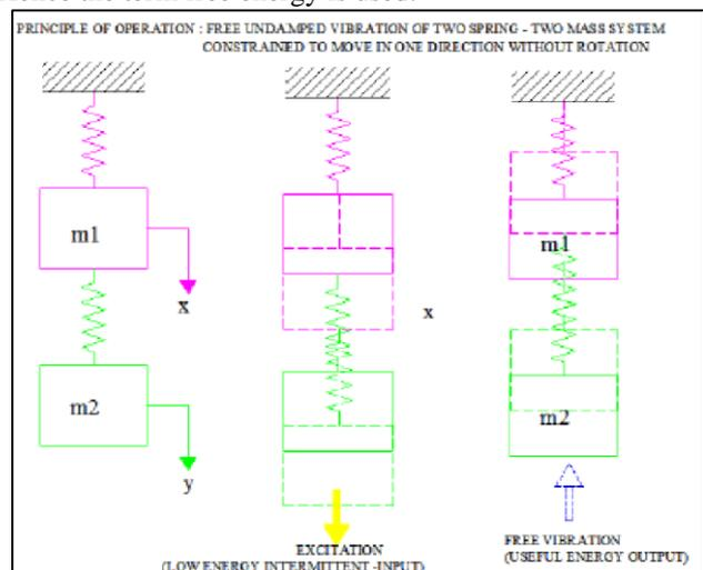
Fig. 2: Two Spring Two Mass Models
