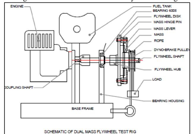
Fig. 4: Schematic of dual mass flywheel test rig
