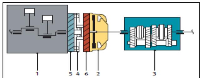
Fig. 1: Principles of Dual Mass Flywheel.
