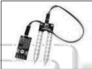
Fig. 1: Soil Moisture Sensor
