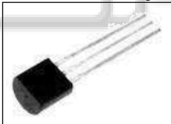
Fig. 2: Temperature Sensor
